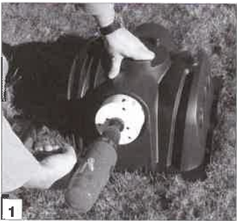
Drill endcap on side or top.
